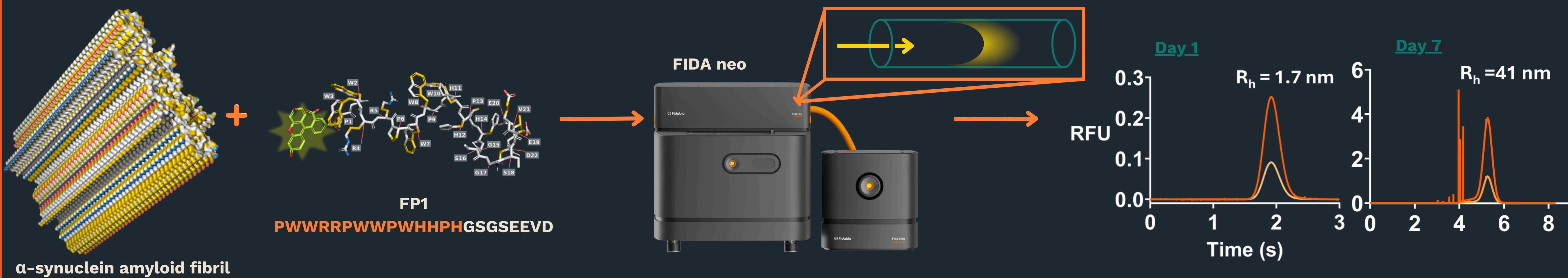
Figure 1: Graphical representation of FibrilRuler method developed in our group, used to study aggregation of \alpha -synuclein. The Amyloid fibril structure is recreated from Cryo-EM analysis of Parkinson's disease patient brains pdb:8fpt. RFU - relative fluorescence intensity
